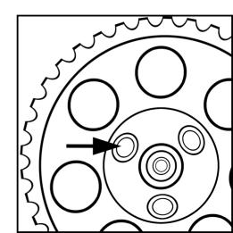
Install the **V 500-1 / V 500-2** assembly to the rear of the engine while hooking the L-shaped bracket over the cover. Leave the center bolt loose until the tool is aligned with the camshaft slots. Once the camshafts are aligned, install the 2 captured bolts and tighten the center bolt. After marking and removing the camshaft sprockets, install the V 500-3 to the front using the previously removed spark plug cover bolts.
