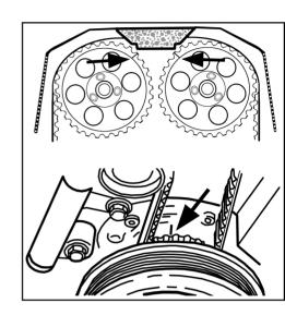
Remove starter and the plug, then install V 500-5.
